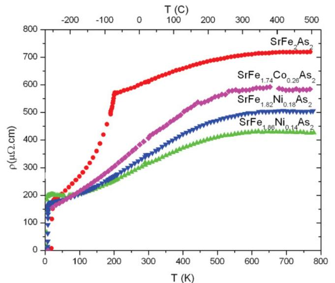
FIG. 2. (Color online) The  $ab$  plane resistivity  $\rho(T)$  up to 800 K for  $\text{SrFe}_2\text{As}_2$  (●),  $\text{SrFe}_{1.86}\text{Ni}_{0.14}\text{As}_2$  (▲),  $\text{SrFe}_{1.82}\text{Ni}_{0.18}\text{As}_2$  (▼), and  $\text{SrFe}_{1.74}\text{Co}_{0.26}\text{As}_2$  (◆) single crystals. The resistivity saturates around 400–700  $\mu\Omega$  cm; the MIR limit is  $\sim 600 \mu\Omega$  cm.
