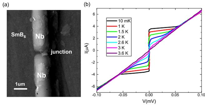
FIG. 1. (a) Scanning electron microscopy SEM image of one of the studied devices, junction-1, made with two Nb leads  $\sim 100$  nm apart on a polished crystal of  $\text{SmB}_6$ . (b) Current-voltage I-V characteristics of junction-1 for a set of temperatures. The supercurrent persists up to 3.6 K.
