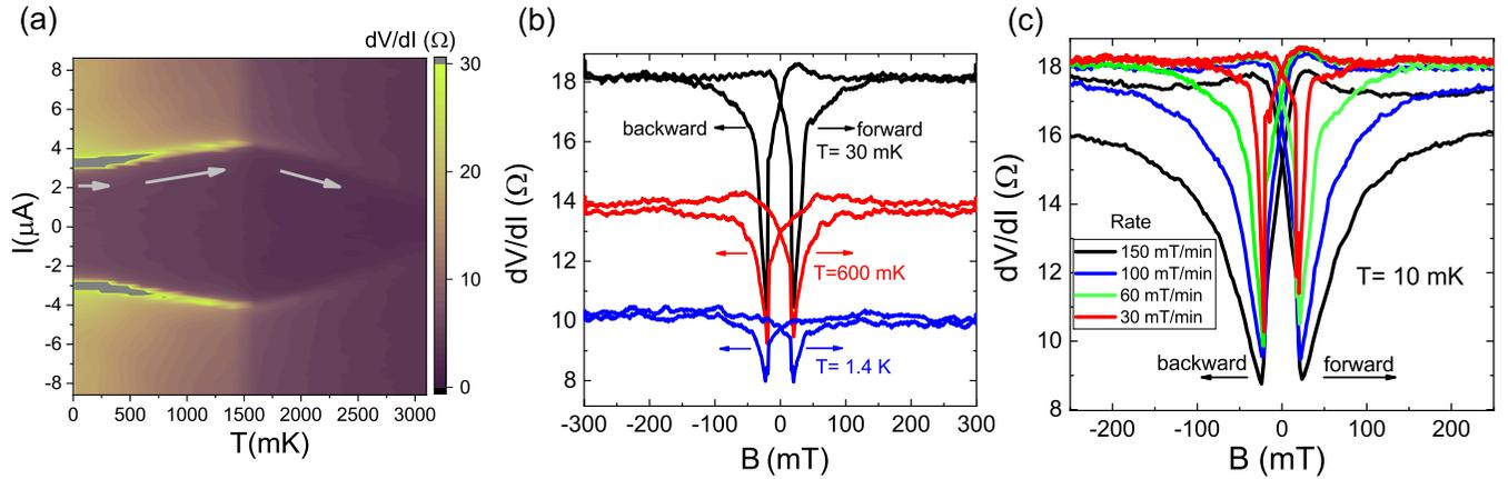
FIG. 4. (a) Color plot of  $dV/dI$  vs bias current as a function of temperature for junction-4. (b) Temperature evolution of hysteresis in normal state resistance with sweep direction for junction-4. (c) Rate dependence of magnetic field hysteresis in normal state resistance of junction-4.
