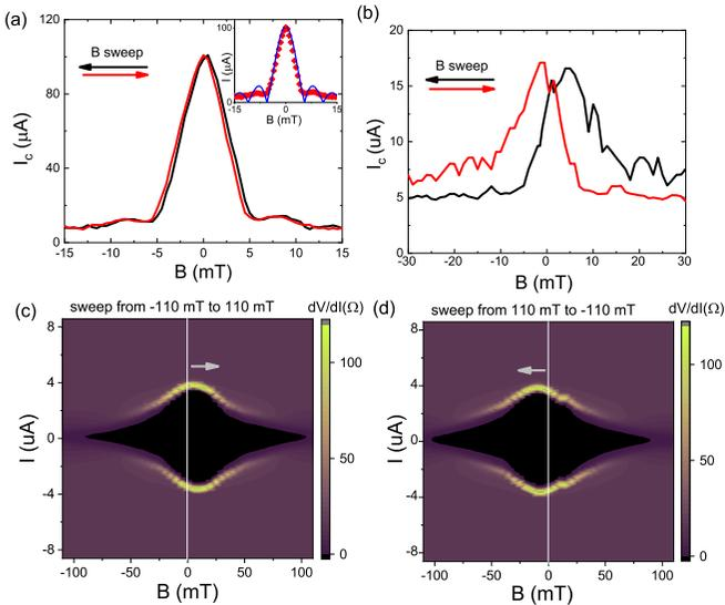
FIG. 3. (a), (b) Magnetic diffraction patterns of the  $I_c$  for junction-3 and junction-2 as the out-of-plane magnetic field is swept in forward and reverse directions. (c) and (d) Color plots of  $dV/dI$  vs bias current as a function of perpendicular magnetic field for junction-1, clearly showing a discernible shift of  $I_c$  with respect to the sweep direction.
