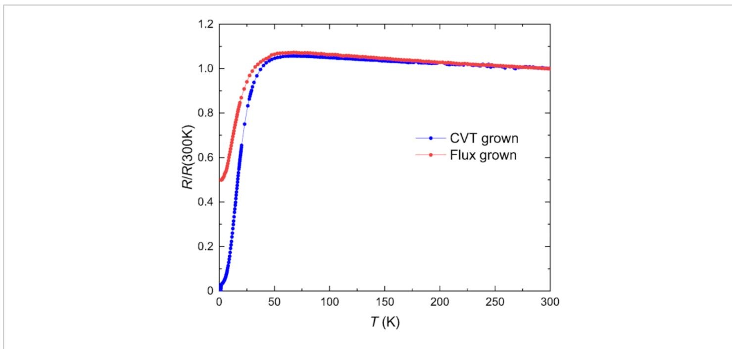
**Figure 3: Normalized electrical resistance data as a function of temperature for both CVT grown and flux grown  $\text{UTe}_2$ .** The flux grown sample has a substantially larger residual resistance, which is a signature of increased crystallographic disorder. [Please click here to view a larger version of this figure.](#)
