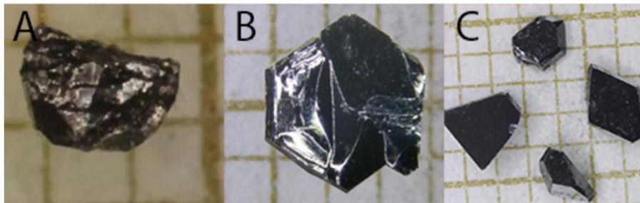
**Figure 1: Photographs of single crystals of  $UTe_2$ .** (A) flux grown and (B-C) CVT grown. The grids are 1 mm. [Please click here to view a larger version of this figure.](#)
