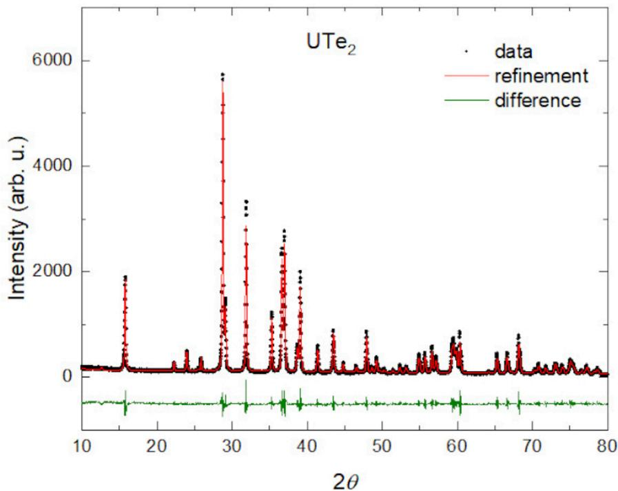
**Figure 2: Powder Xray diffraction data of CVT grown  $UTe_2$ .** The data shows the good quality of the sample with no visible peaks from impurities. [Please click here to view a larger version of this figure.](#)
