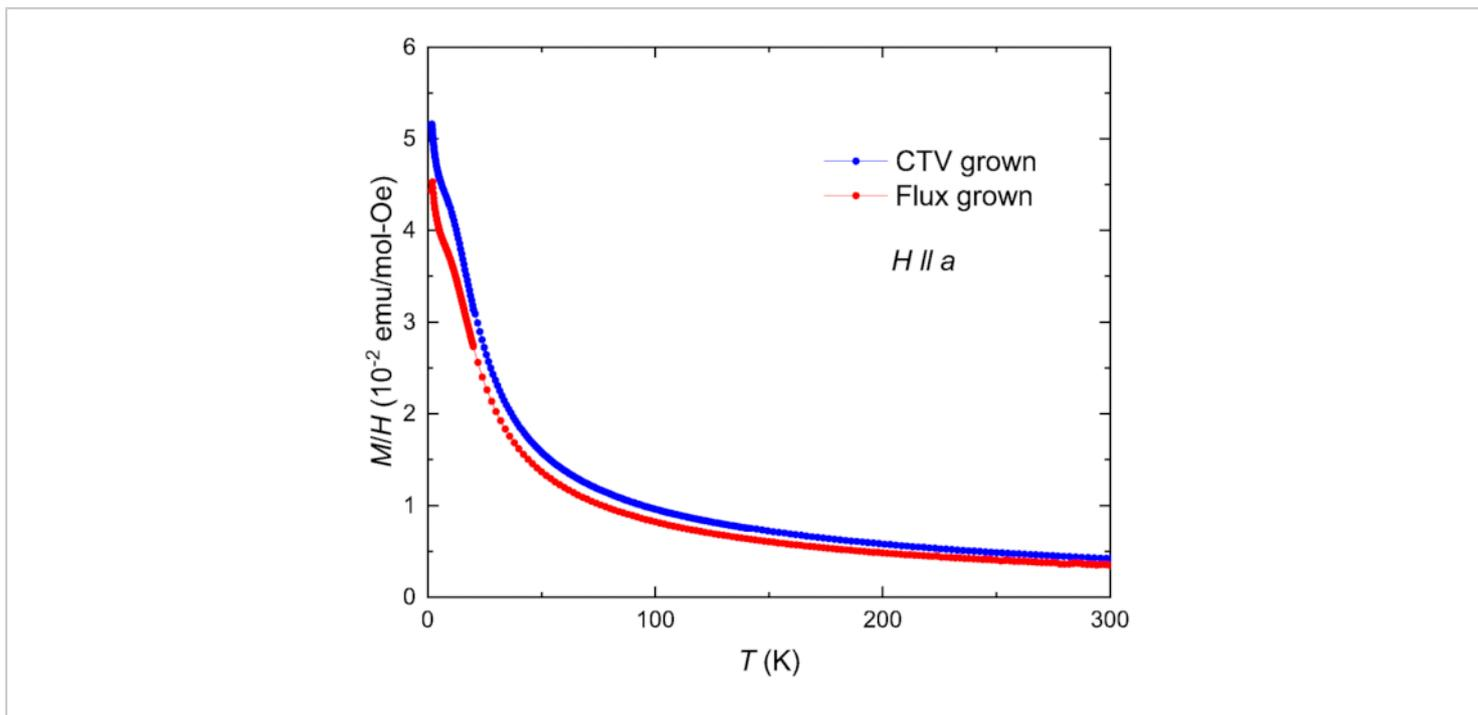
**Figure 4: Magnetic susceptibility, or magnetization normalized to applied magnetic field, as a function of temperature for both CVT grown and flux grown  $UTe_2$ .** The samples show similar behavior, including a characteristic kink at approximately 10 K. A magnetic field  $H = 1000$  Oe is applied parallel to the crystallographic a-axis. [Please click here to view a larger version of this figure.](#)
