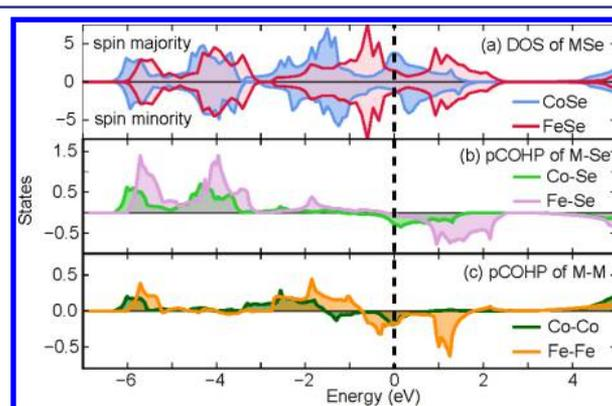
**Figure 10.** (a) The spin-polarized electronic density of states (DOS) of FeSe and CoSe. (b) The partial crystal orbital Hamilton population (pCOHP) to describe the  $M$ -Se bonding and antibonding interactions. (c) The pCOHP for  $M$ - $M$  interactions. In (b) and (c), positive and negative states represent bonding and antibonding interactions, respectively.
