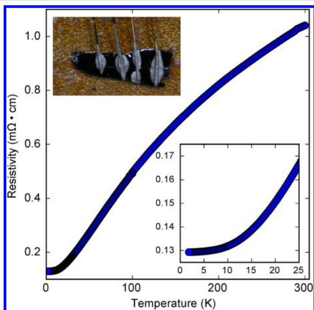
**Figure 8.** Temperature dependent electrical resistivity of CoSe measured on a single crystal. CoSe displays metallic behavior at high temperature with a slight deviation in slope around  $10$  K (inset), close to the ferromagnetic transition temperature.
