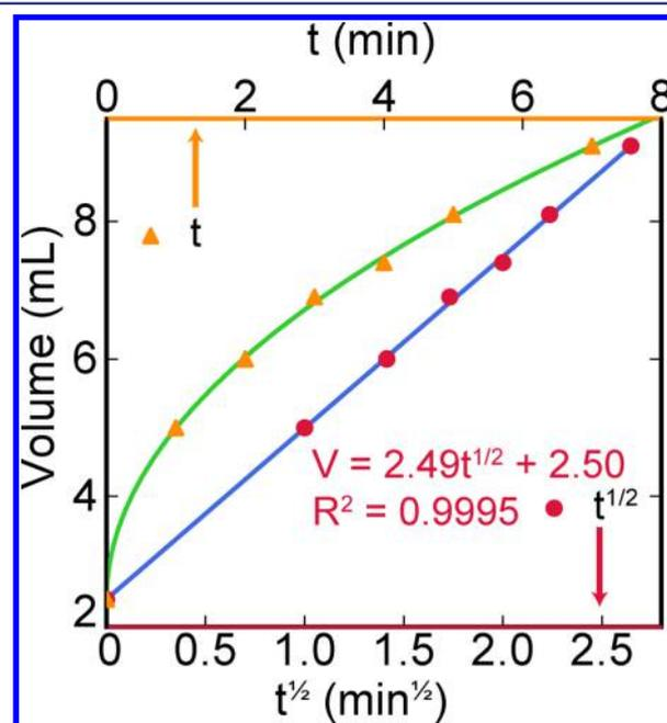
**Figure 2.** Volume of hydrogen generated during a deintercalation reaction of  $\text{KCo}_2\text{Se}_2$  vs time  $t$  and  $t^{1/2}$  leading to the preparation of pure CoSe. For this reaction,  $t = 0$  is the point when water flow was observed from  $\text{H}_2$  generation. The lines drawn represent a least-square fit of the data.
