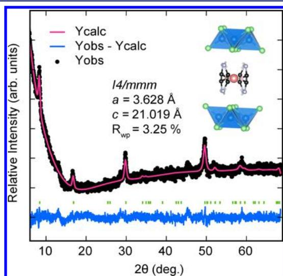
**Figure 9.** Powder X-ray diffraction patterns of ground polycrystalline  $\text{Li}(\text{C}_2\text{H}_8\text{N}_2)\text{CoSe}$  collected at room temperature. Refinement of the  $\text{Li}(\text{C}_2\text{H}_8\text{N}_2)\text{CoSe}$  structure in the body-centered tetragonal group ( $I4/mmm$ ). Tick marks represent the corresponding phase.
