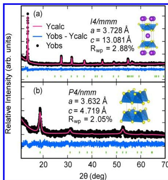
**Figure 4.** Powder X-ray diffraction patterns with  $\text{Cu K}\alpha$  radiation of (a)  $\text{KCo}_2\text{S}_2$  and (b)  $\text{CoS}$  collected at room temperature. Tick marks representing the corresponding tetragonal phases are shown below the calculated, observed, and differences curves from Rietveld analysis for (a) and Pawley fit for (b).
