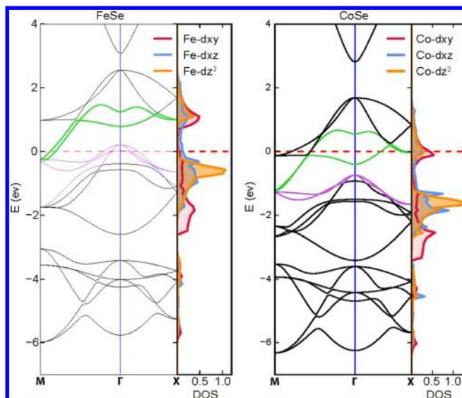
**Figure 11.** Band structure along three different directions and the corresponding partial DOS of 3d states for FeSe and CoSe. Purple and green lines in the band structure indicate bands crossing the Fermi-level close to the  $\Gamma$  and  $M$  points, respectively.
