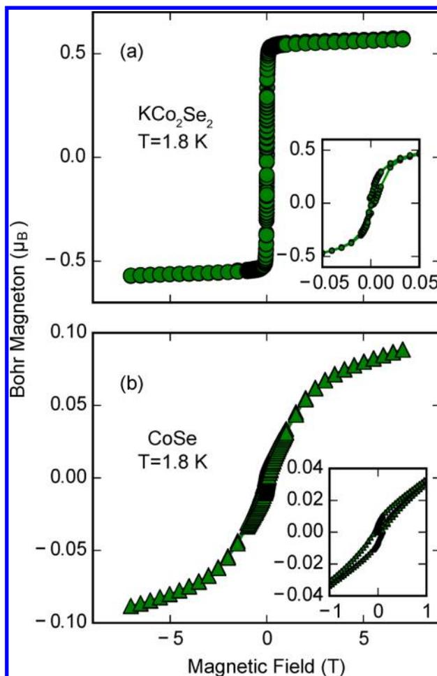
**Figure 6.** Isothermal magnetization vs applied field  $H$  for (a)  $\text{KCo}_2\text{Se}_2$  and (b)  $\text{CoSe}$  at 1.8 K. Both  $\text{KCo}_2\text{Se}_2$  and  $\text{CoSe}$  show hysteretic behavior indicating ferromagnetic ordering.
