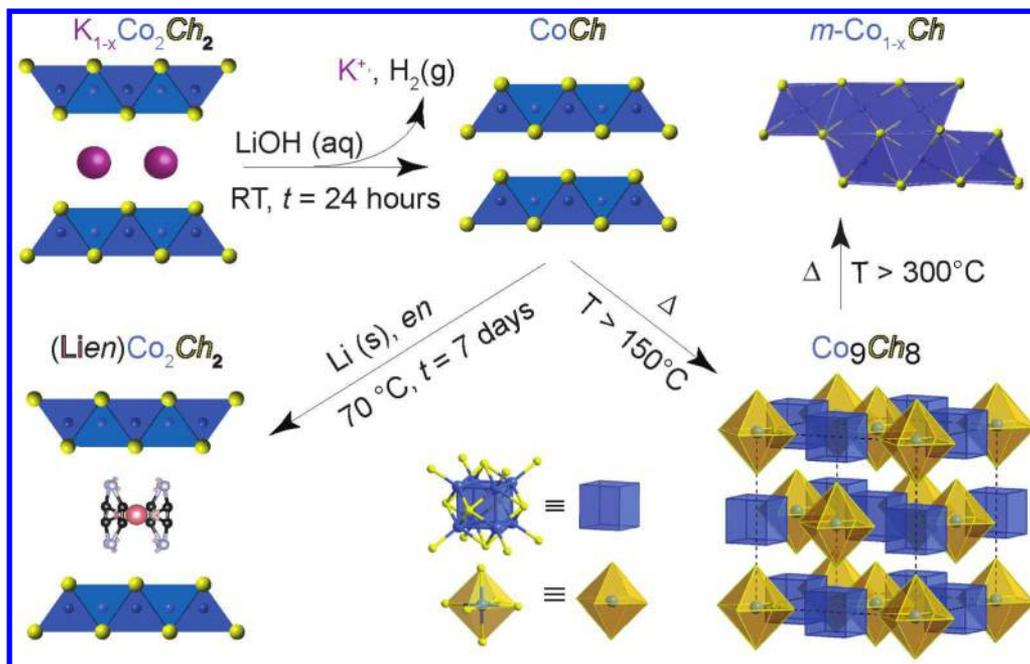
**Figure 1.** Reaction schemes for the manipulation of cobalt chalcogenides. From the thermodynamically stable  $K_xCo_2Ch_2$  phases, we prepare metastable tetragonal  $CoCh$  and  $(Lien)CoCh$  where  $en$  = ethylenediamine. Upon applying heat to the metastable phases, pentlandite ( $Co_9Se_8$ ) is prepared followed by the NiAs-derivative  $m-Co_{1-x}Ch$ .
