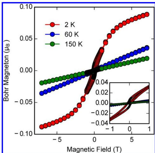
**Figure 7.** Isothermal magnetization vs applied field  $H$  for CoSe at  $T = 2, 60,$  and  $150$  K. While the  $2$  K data displays hysteresis with some blocking, the  $60$  and  $150$  K data indicate paramagnetic behavior. The inset shows a zoomed region emphasizing the disappearance of hysteresis at higher temperatures.
