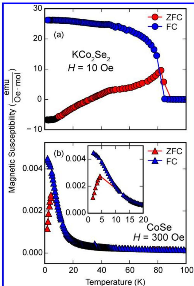
**Figure 5.** Magnetic susceptibility of (a)  $\text{KCo}_2\text{Se}_2$  and (b)  $\text{CoSe}$ , vs temperature measured in applied field of 10 and 300 Oe, respectively. (a)  $\text{KCo}_2\text{Se}_2$  displays a ferromagnetic transition at  $T_C = 82$  K and (b)  $\text{CoSe}$  a  $T_C = 10$  K; the inset shows zoomed-in region near  $T_C$ .
