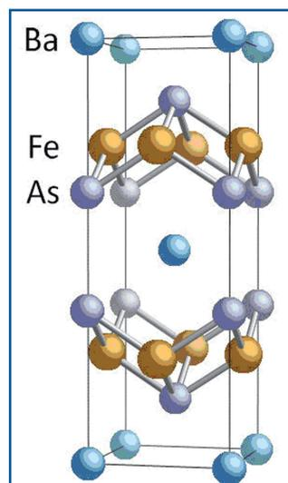
Fig. 1 Atomic arrangement of the iron-based superconducting compounds with ThCr<sub>2</sub>Si<sub>2</sub>-type structure, shown for the intermetallic material BaFe<sub>2</sub>As<sub>2</sub>. The FeAs-type tetrahedrally coordinated layers are the key structural ingredient in all iron-based superconducting materials known to date.
