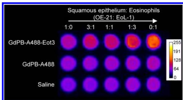
**Figure 7.** Nanoparticles allow quantitative detection of eosinophils by MRI at 3 T. (A) MRI phantom of GdPB-A488-Eot3, GdPB-A488, and saline added to suspensions containing varying ratios of squamous epithelial cells (OE-21) and eosinophils (EoL-1) (OE-21:EoL-1 ratios used were 1:0, 3:1, 1:1, 3:1, and 0:1). The amounts of the nanoparticles added are constant for all samples.
